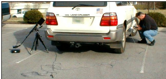
Below is a picture of the complete ORION remote system including a tri-pod and an ORION with a toolkit.
